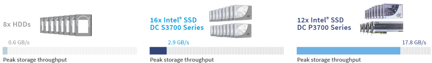
Figure 2: The peak disk throughput in GB per second for each solution. Larger numbers are better.
