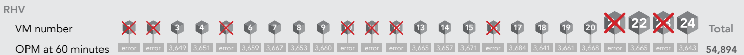
Figure 10: RHV powered on only two new VMs and restarted seven of the original VMs. A red X represents a failed or automatically restarted VM.
