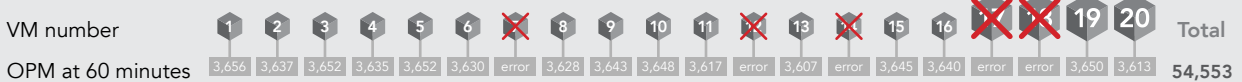
Figure 7: RHV powered on only two new VMs and restarted three of the original VMs. A red X represents a failed or restarted VM.
